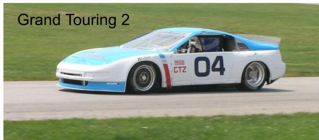
deep. The Grand Touring cars use tube frame chassis and the bodywork has been modified to permit super-wide racing slicks to fit under the fenders. The Production cars
