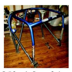
**Roll Cage for Bugeye Sprite** Removed from a bugeye that has been raced since the early seventies. Never been crashed, will fit similar chassis. Some welding needed to re-install it and four holes in the skin are needed but the rest is bolt in. 13/4" dia. 1/8" wall mild steel tubing. Professionally heli-arc welded. \$500.00 If interested call Harold Hammerly 317-507-1101
